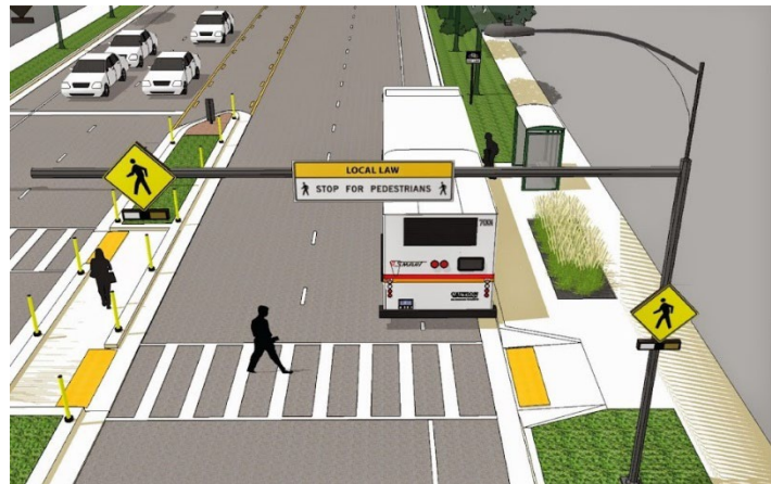
Figure 16: Source: The Greenway Collaborative Inc. – Best Practice Guidelines: Mid-Block Crosswalks for arterial five lane roadways
